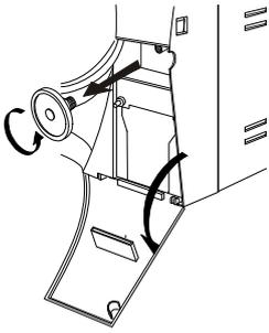
When it is due to be changed, or when you notice visible clogging of the filter (indicated by a color markedly tending towards gray) unscrew the bacteriological filter from its support and replace it with a new one by screwing it all the way down on the connector on the front of the machine.
