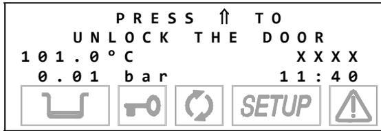
Press the ↑ key to unlock the door lock mechanism; the following message appears:
