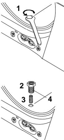
With use, various residues will probably tend to accumulate inside the filter, obstructing the lower drain tube over time.
