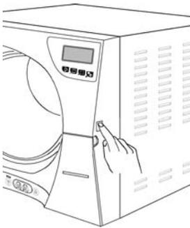
The system is **RESET** in two alternative ways, depending on the alarm that occurred (see the **Alarm Code List** further below in this appendix):
