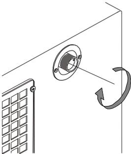
1. Access the safety valve located on the rear of the machine.
