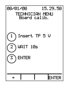
Now set the calibration tool switch to 5 V (position 1). Wait for at least 10 seconds and press ENTER.
