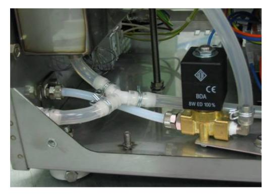
• Insert the *probe support E* in the silicon pipe and fasten the ends with the pipe clamps provided. Connect to the pins using the appropriate screws and ready to use and clamped blue cables with eyelets to the *filler* 14. Clamp *probe support E* to the supplied support screwed into the *slit J*, making sure there is no contact between the pins and other parts of the steriliser.
