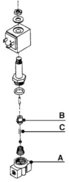
Replace the solenoid valve when time or number of cycles shown in the Scheduled service table is exceeded (see USE AND MAINTENANCE MANUAL, chapter MAINTENANCE). Proceed as follows if cleaning is required:
