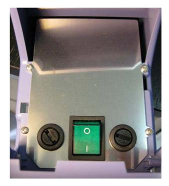
Fit the frame (C) on the control panel (P) with the four screws previously removed • from the lid  $(\mathbf{R})$ .
