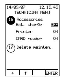
Select Accessories (option 16) and press ENTER. The external charge value (ON/OFF) will appear. Press  $\uparrow\downarrow$  to change the value, press ENTER to confirm and move to the next option.
