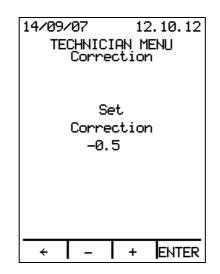
Press +/- to enter the correction which will change the temperature shown on the display. Press ENTER to confirm.
