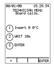
Disconnect the connector from the electronic power board corresponding to the temperature probe you want to calibrate: disconnect connector CN12 for sensor PT1, connector CN13 for sensor PT2 or connector CN14 for sensor PT3.
