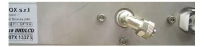
• Replace the *automatic water inlet pump* **46** and the connection pipes with the *solenoid valve EV7* (mounted on its support and with the outlet hose holders and the inlet L-joint) and the pipes supplied. Use the teflon pipe to connect the internal joint on the back of the steriliser with the *solenoid valve EV7* (inlet 1) and use the silicone pipe to connect the *solenoid valve EV7* (outlet 2) to the *clean water tank* **10**.
