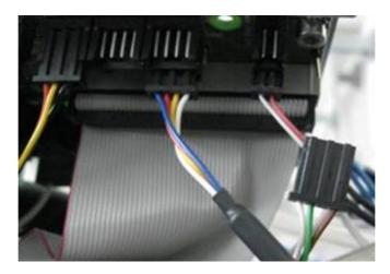
Connect the 4 pin cable of the calibration tool to connector CN11 of the power board. Set the calibration tool switch to 0 V (position 2):
