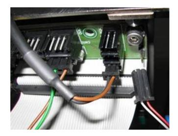
Connect the 2 pin cable of the calibration tool to connector CN12, CN13 or CN14 of the power board. Put ON the switch number 1 of the temperature selector, which corresponds to a 1000 Ohm sample coil, corresponding to 0°C:
