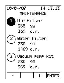
The remaining days and cycles and the last three replacements are shown for each item with the date of intervention and the total number of cycles when the replacement was performed.
