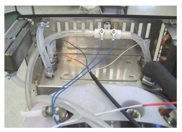
The presence of fouling or lime scales may create electric continuity between tank metal and level probe rod and consequently read the presence of liquid in the tank when the tank is empty. If messages and alarm appear after emptying the tanks, remove the probes and clean the probes carefully as follows:
