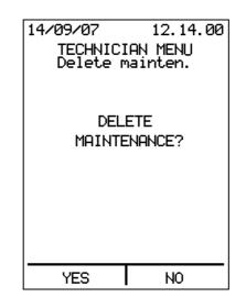
Press YES to delete all maintenance interventions performed on the steriliser from the machine memory and reset the remaining day and cycle counters for all components. Press NO to keep the maintenance log and go back to the Technician Menu.
