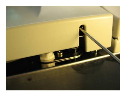
Unlocking tool **37** must be fully inserted. Open the door without forcing it, remove *unlocking tool* **37** and open the handle completely.
